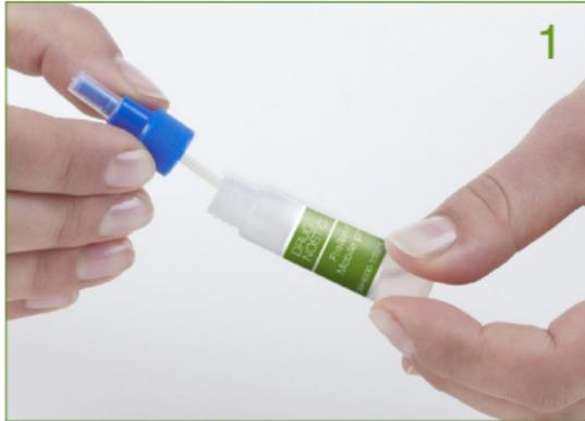
Take the bottle of mobile phase out of the pack. Unscrew the blue cap. Put the substance to be tested in the bottle and close it again. Leave it standing (not horizontal) at room temperature overnight, or for about 12 hours.
