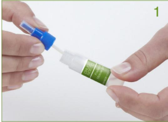
Take the bottle of mobile phase out of the pack. Unscrew the blue cap. Pour one to three drops of the suspicious liquid into the opened bottle. Screw the cap back on and shake the bottle.
