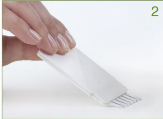
Wipe over one or more suspicious surfaces with the free end of the test strip.
